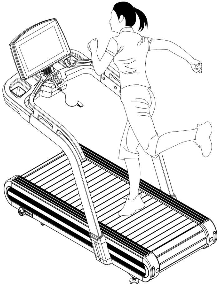
23 When you are ready for running, please do not stand on the running belt. Before starting the machine, turn on the power. Put your hands on the side handrail and stand on the protection bar at both sides. And then press "START", when the motor is working in low speed, move your feet to the running belt to start running.
